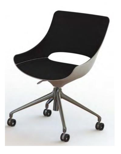
The chair shell is a complex injection moulding that was carefully developed through many iterations, from card and paper models, CNC foam and fiberglass prototypes prior to investment in tooling. Recycled and recyclable materials are used throughout, using Computer Aided Design to minimise their volume without compromising the structure.
