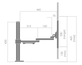
Add-on Arm allows for screens to be mounted at the same height or independantly adjusted Note: Maximum reach is dependant upon screen size.
